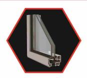
The Prime Window system, designed for projects where less profile visibility and maximum view are desired, is a concealed sash system where all visible exterior widths can be made 55 mm. With a 34 mm glass fiber-reinforced polyamide barrier and a total frame depth of 92 mm, the system allows for the use of desired large openings and different glass combinations.
